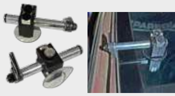
SET OF ASSEMBLY JIG ensures the distance between the windshield and the frame of the car, precision to the mm, 10 wedges of 1mm each
