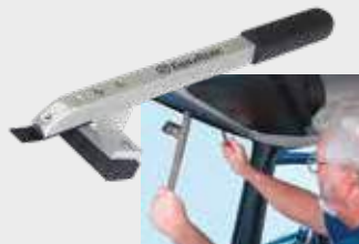
FOOTLOSE RUBBER GASKET RELEASE TOOL for wide windshield seals, insert the tip between the glass and the window and press slightly outward to remove the seal.
