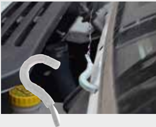
HOOK to attach the wire to a fixing part of the body of the car
