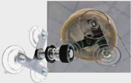
PIANO WIRE DISPENSER mounted on a suction cup, is positioned on the wind- shield and allows the rope to be inserted around the windshield in a completely autonomous way.
