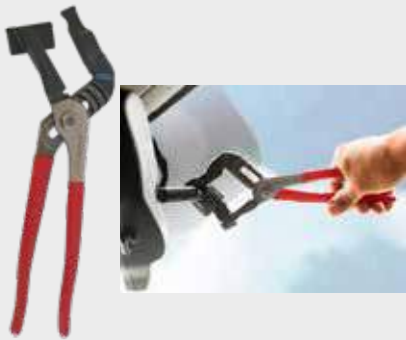
REARVIEW MIRROR INSTALLER for spring-loaded mirrors, set the upper jaw against the rearview mirror, put the nylon block against the rearview mirror mounting bracket and squeeze the handles
