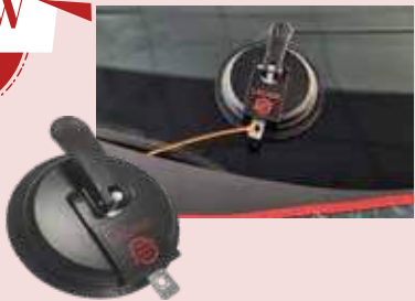
ANCHOR CUP for holding the windscreen gasket cutting cord
