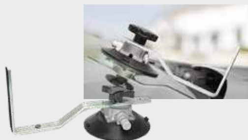
WINDSHIELD ADJUSTMENT SUCTION CUP with protective felt, position the suction cup, the stop must be wedged on the hood, once the windshield is glued it is automatically well positioned
