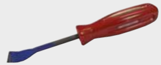
"CHRISTMAS TREE" MOULDING REMOVER can easily be inserted under the moulding, does not damage the profile. The curvature guarantees the leverage effect to remove the clips.
